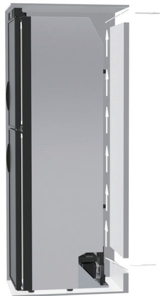
EXTERNAL COOLING CYCLE INSTALLATION
